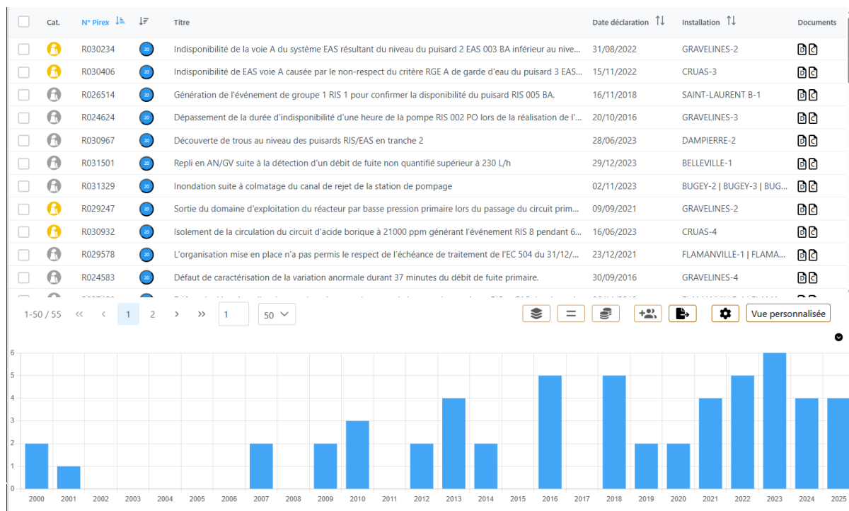
Figure 1-1: Histogram of safety events concerning water level measurement in the sumps in France since 2000
